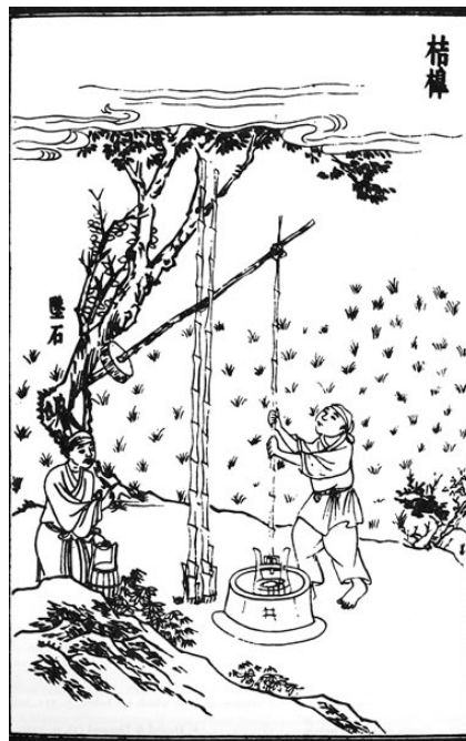
〈Figure 12〉 Swape (or “well-sweep”) technology employs a counter-balanced bailing bucket that saves time and energy in agricultural production.
